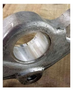
The side of the bore with the flat side should face down when pressing in the bushings.
