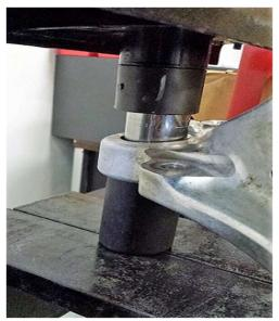
Press out the stock bushing using an appropriate bushing press and driver. As shown, we used a 1 1/8 inch socket as the driver. Keep the flat side of the arm facing down.
