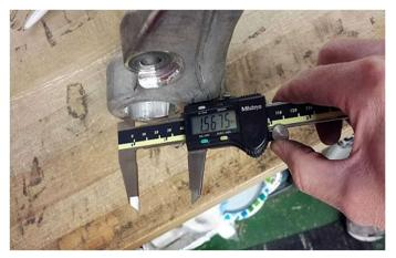
Check and clean the bores, file down any nicks in the bore as necessary.
